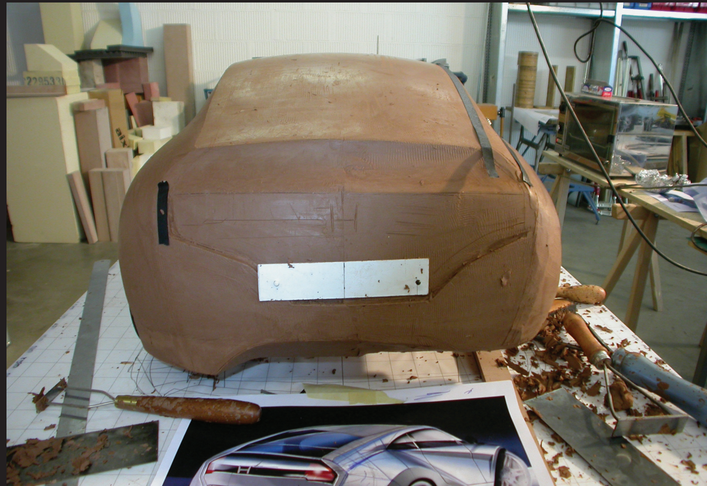
Clay Modelling: 1:4 exterior shape definition Clay Modellbau: 1:4 Exterieur Formfindung
